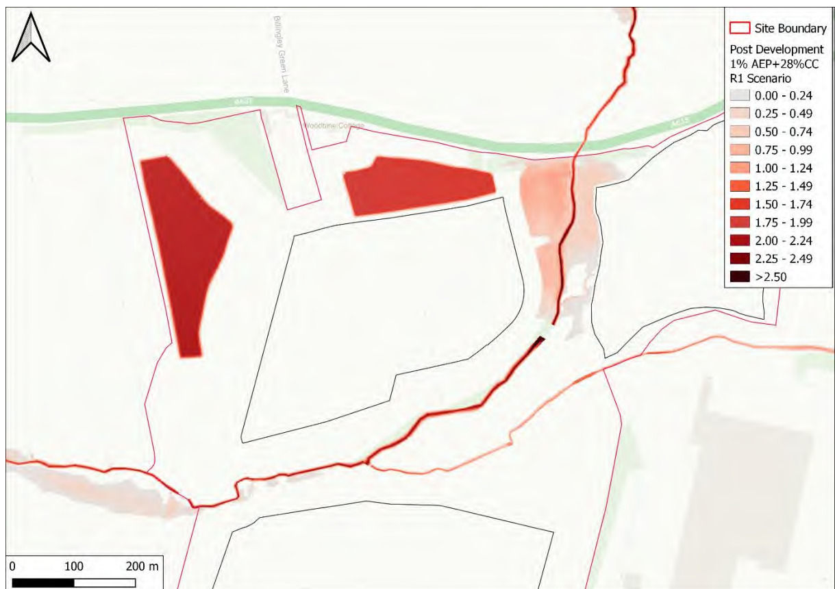
Figure 37: Post Development 1% AEP+28%CC (1 in 100-year plus Climate Change) with a 50% blockage to the Carr Dike Culvert
