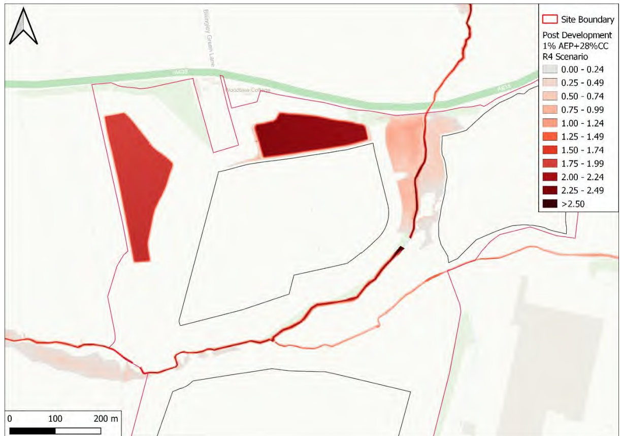
Figure 40: Post Development 1% AEP+28%CC (1 in 100-year plus Climate Change) with a 50% blockage to the Culvert between FCA and FSA
