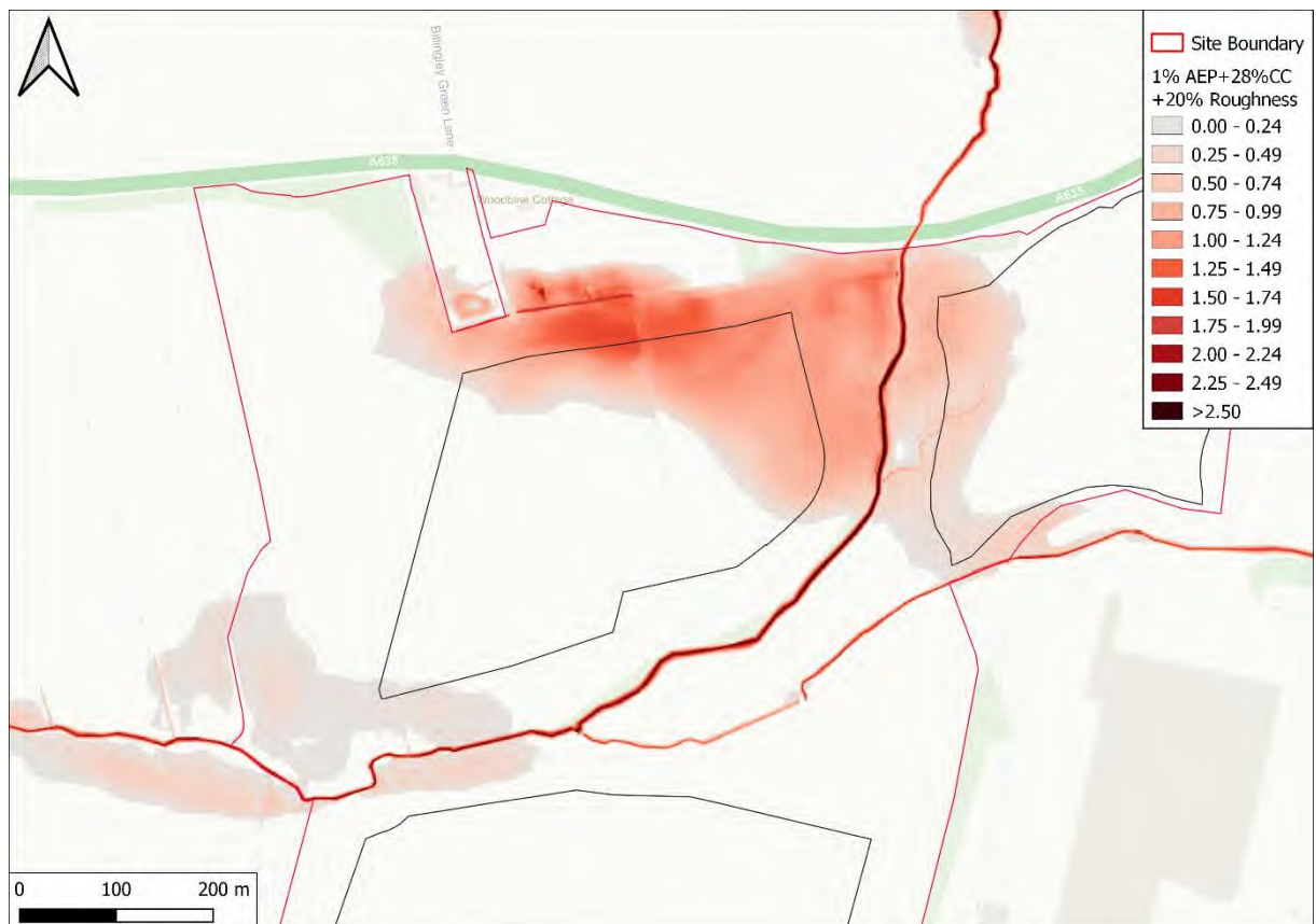
Figure 26: 1% AEP+28%CC (1 in 100-year plus Climate Change) with a 20% increase in Manning's Roughness Values
