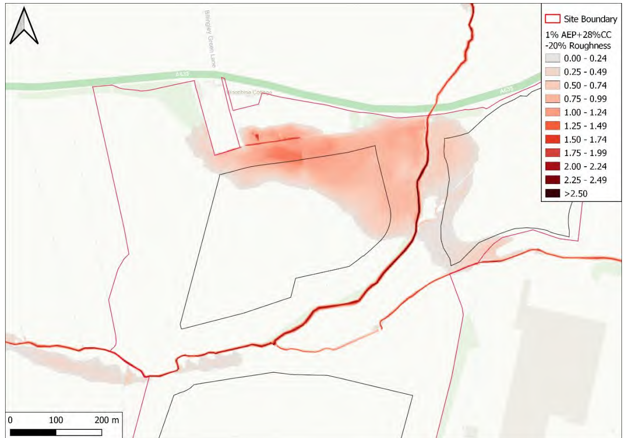
Figure 27 1% AEP+28%CC (1 in 100-year plus Climate Change) with a 20% decrease in Manning's Roughness Values
