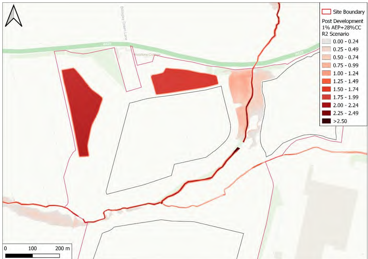
Figure 38: Post Development 1% AEP+28%CC (1 in 100-year plus Climate Change) with a 50% blockage to the Highgate Lane Dike Culvert
