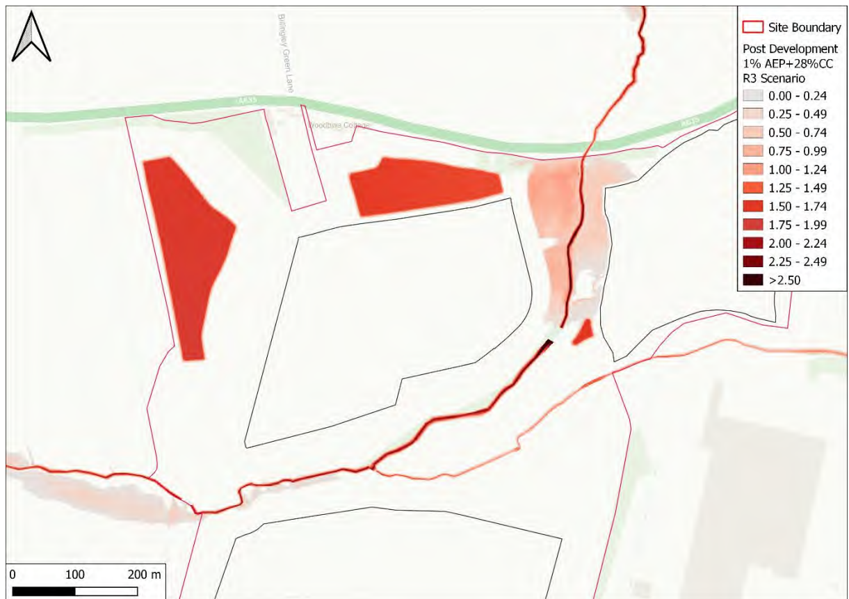
Figure 39: Post Development 1% AEP+28%CC (1 in 100-year plus Climate Change) with a 50% blockage to the FCA Culvert
