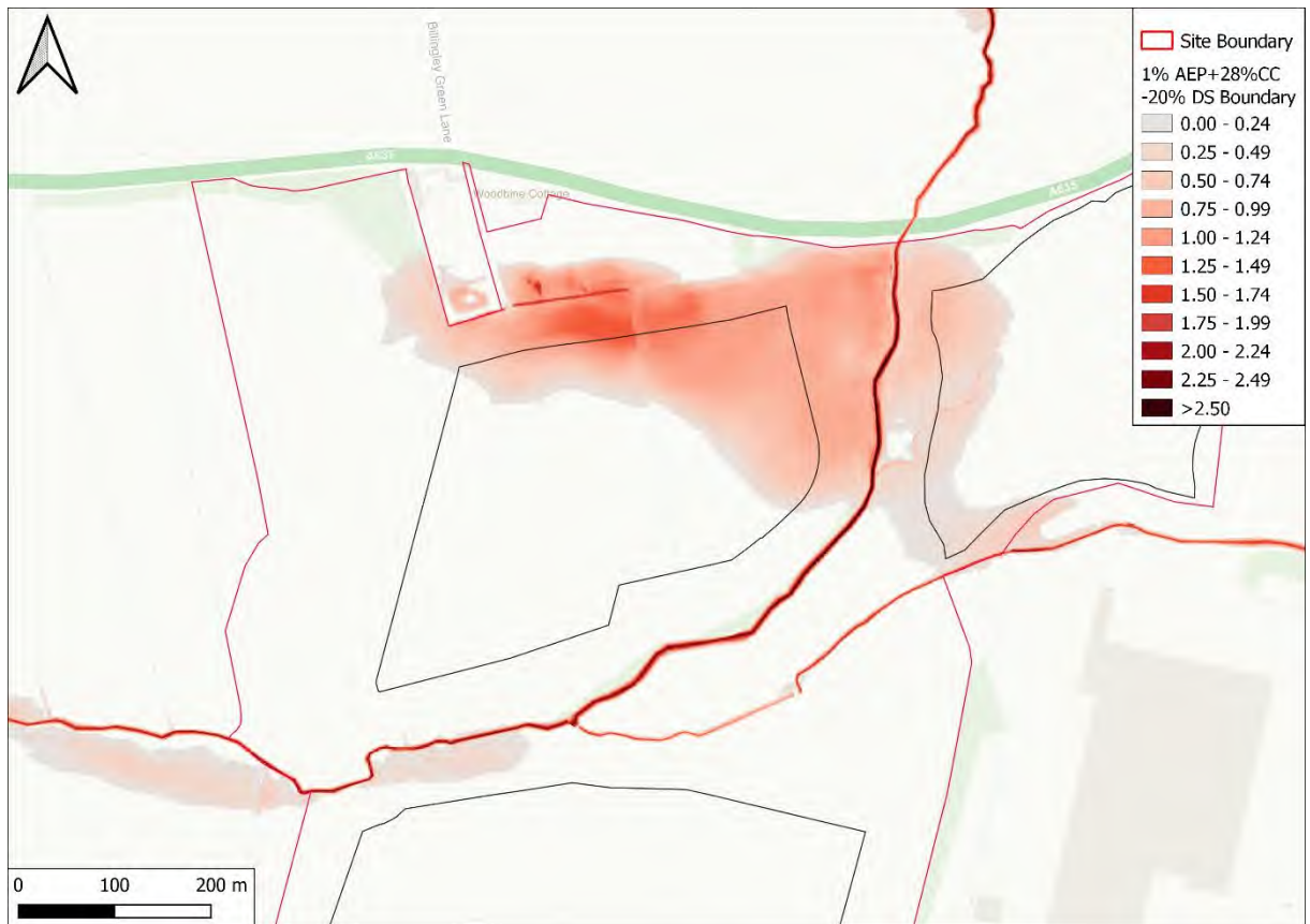
Figure 29: 1% AEP+28%CC (1 in 100-year plus Climate Change) with a 0.3m decrease in Downstream Boundary Level
