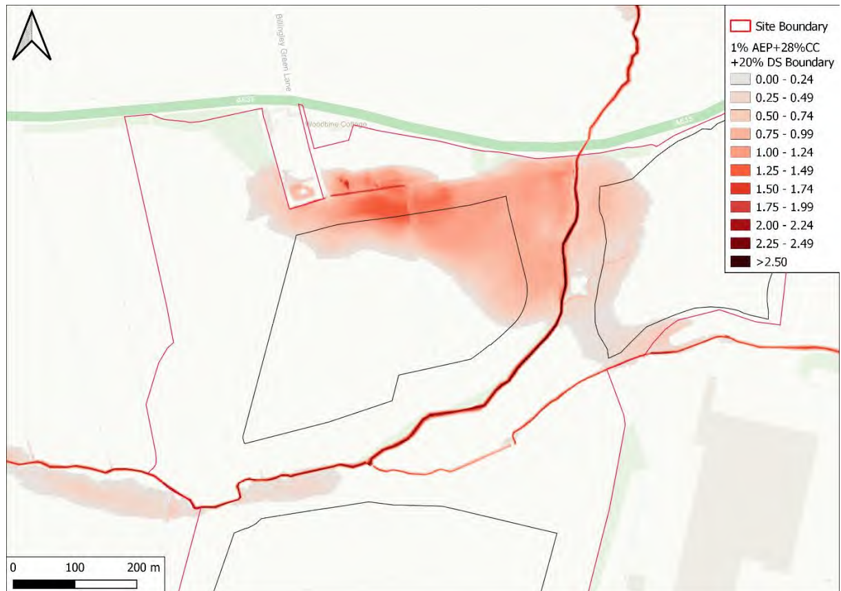
Figure 28: 1% AEP+28%CC (1 in 100-year plus Climate Change) with a 0.3m increase in Downstream Boundary Level
