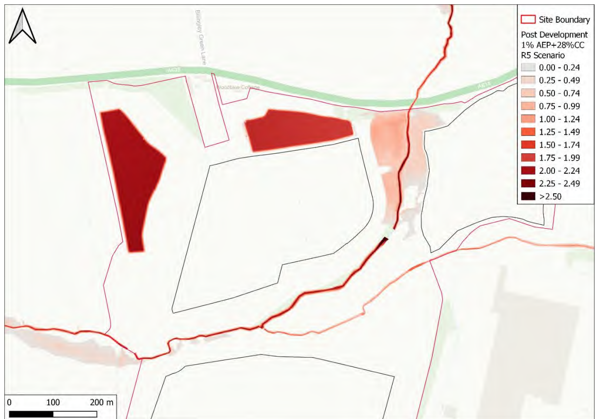
Figure 41: Post Development 1% AEP+28%CC (1 in 100-year plus Climate Change) with a 90% blockage to the FSA Culvert
