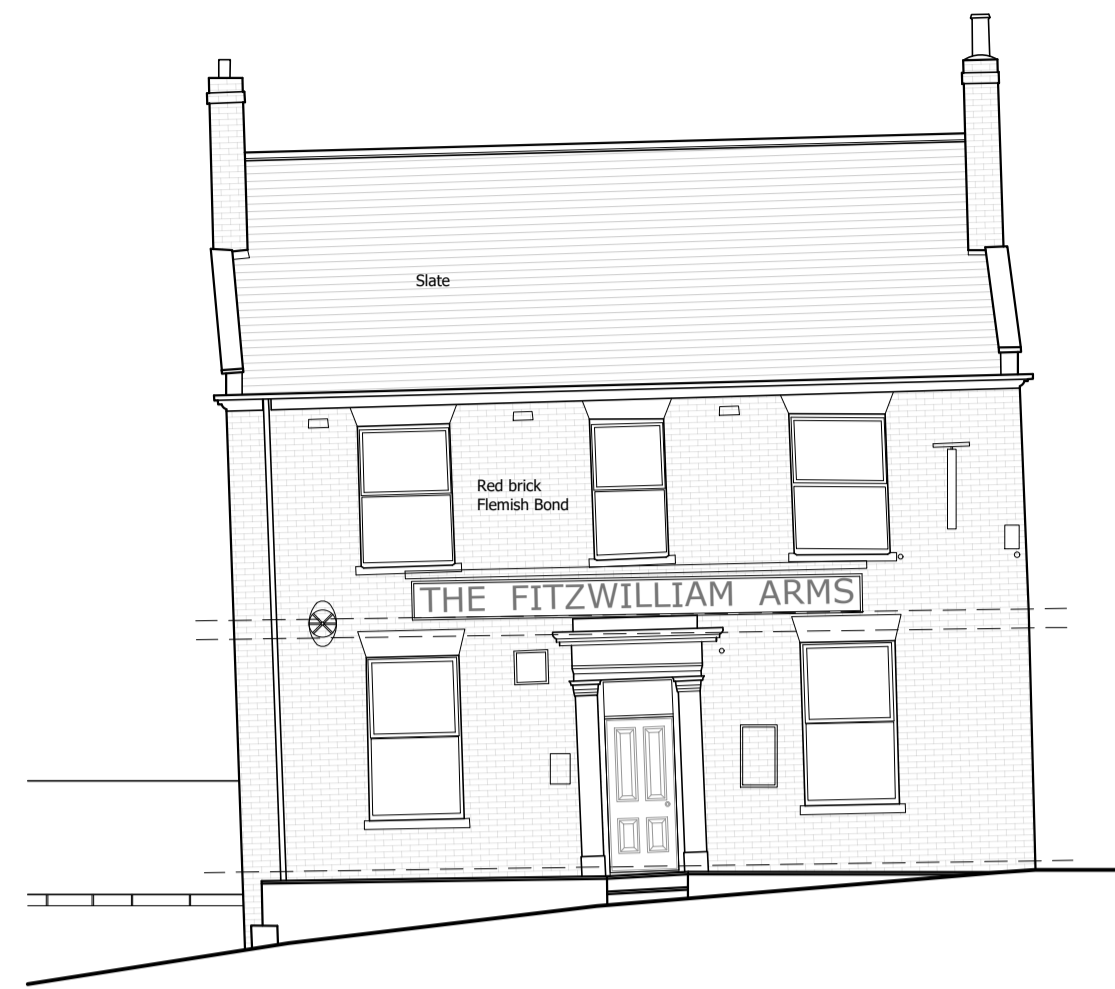
EXISTING FRONT ELEVATION (EAST) Scale - 1: 100 @ A1
