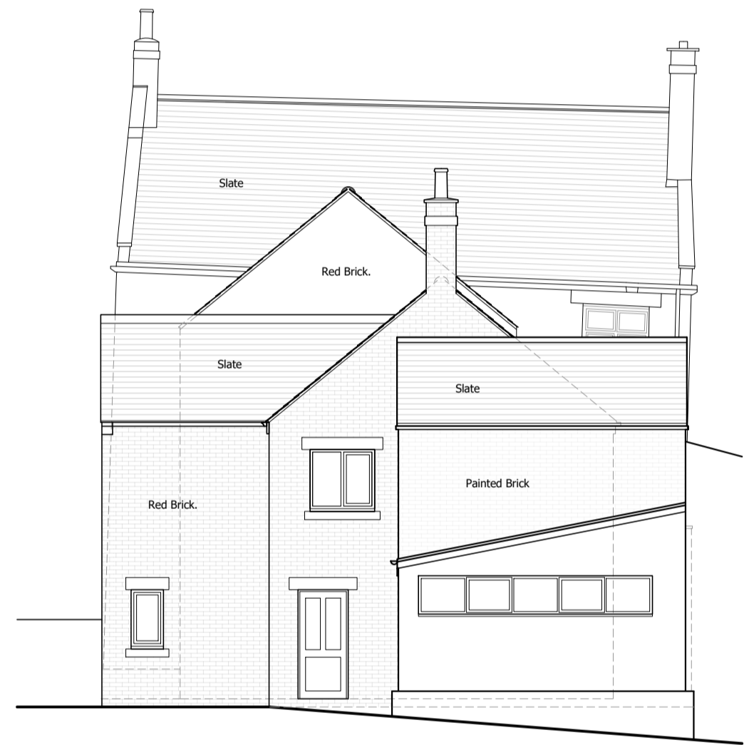
EXISTING REAR ELEVATION (WEST) Scale - 1: 100 @ A1
