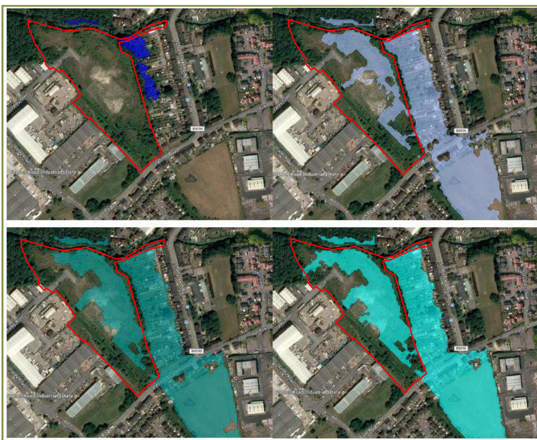
Top Left: 1 in 100-year Top Right: 1 in 100-year+30%CC Bottom Left: 1 in 100-year+50%CC Bottom Right: 1 in 1000-year
