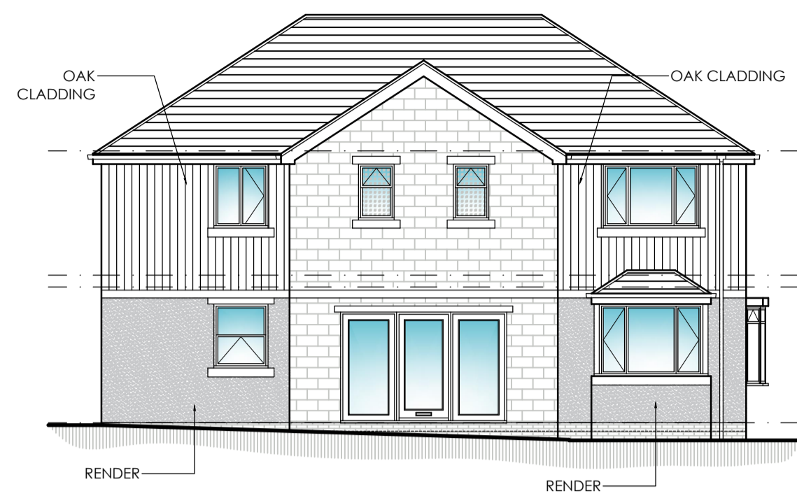
PROPOSED FRONT ELEVATION SCALE 1:100
