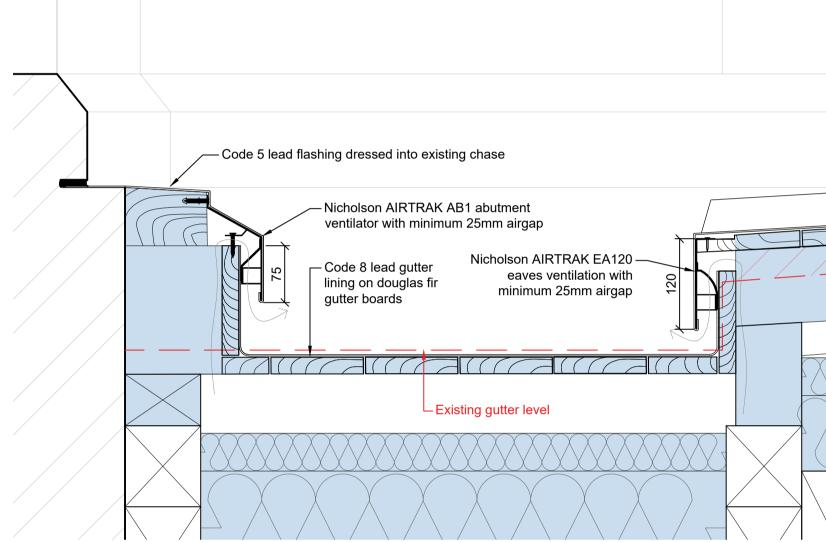
Detail 1: Section through proposed lead gutter
