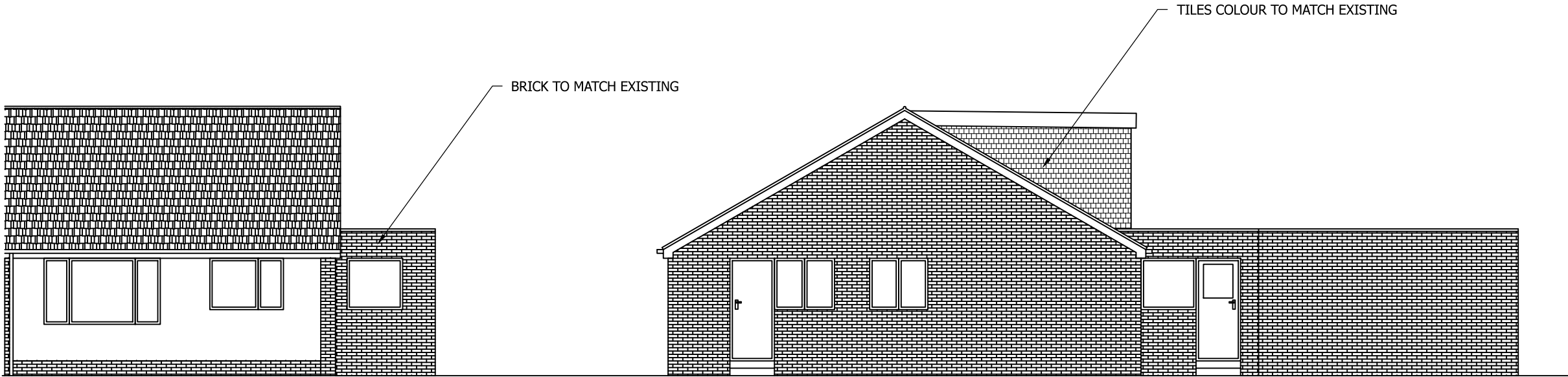
PROPOSED FRONT ELEVATION SCALE 1:100 AT A3
