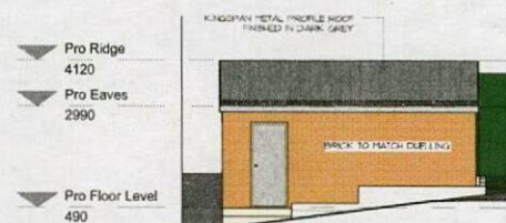
Side Elevation (East Facing) 1 : 100
