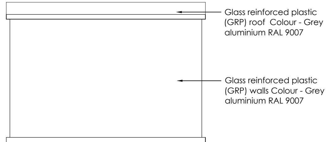
Proposed North Side Elevation 1:50 @ A3
