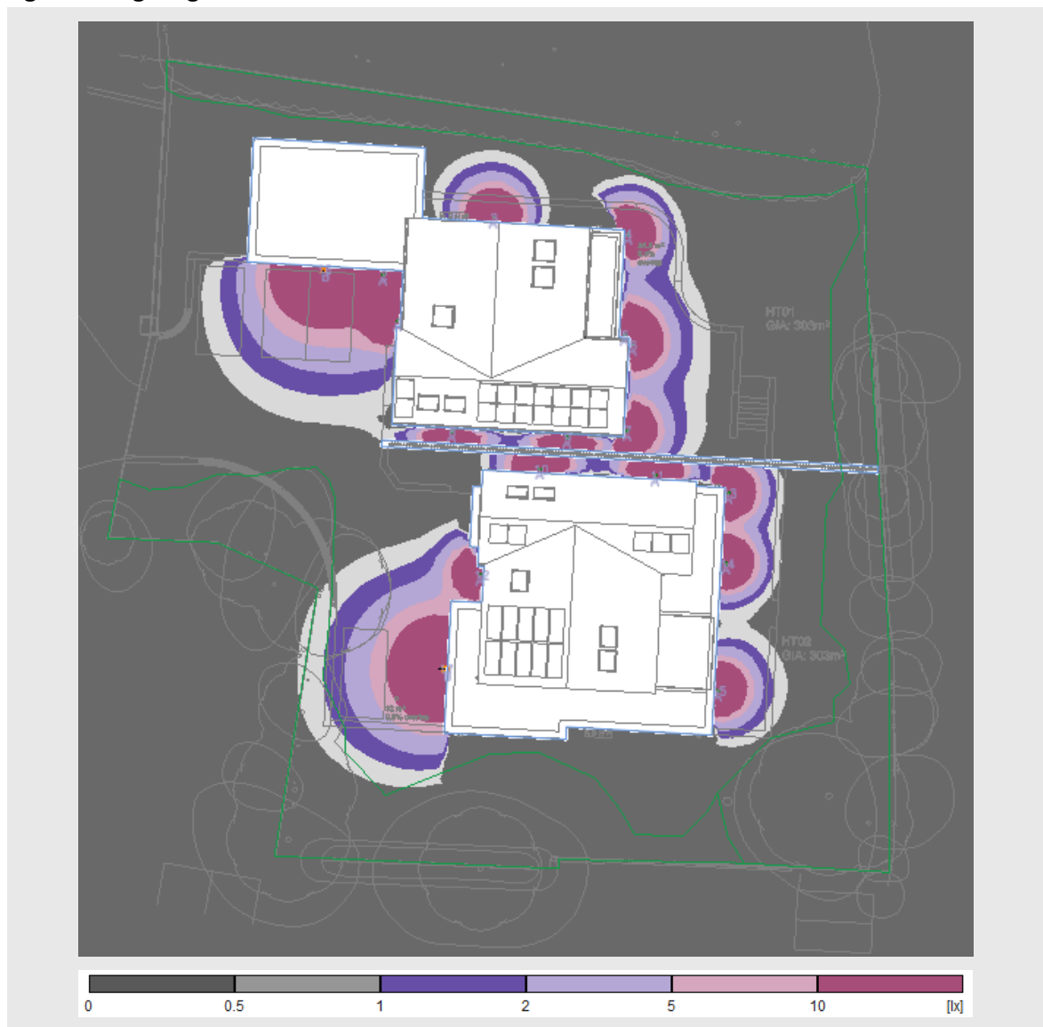
Figure 7.1 Lighting model false colour view - measurements in lux
