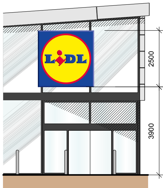
Wall Mounted Signage Height Scale 1:100 @ A4
