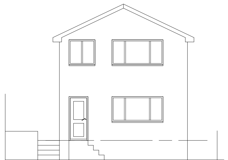
EXISTING FRONT ELEVATION 1:100
