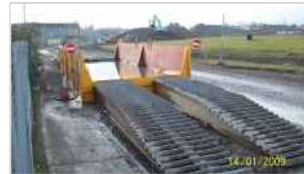
Proposed Wheel Wash Scale 1:150
