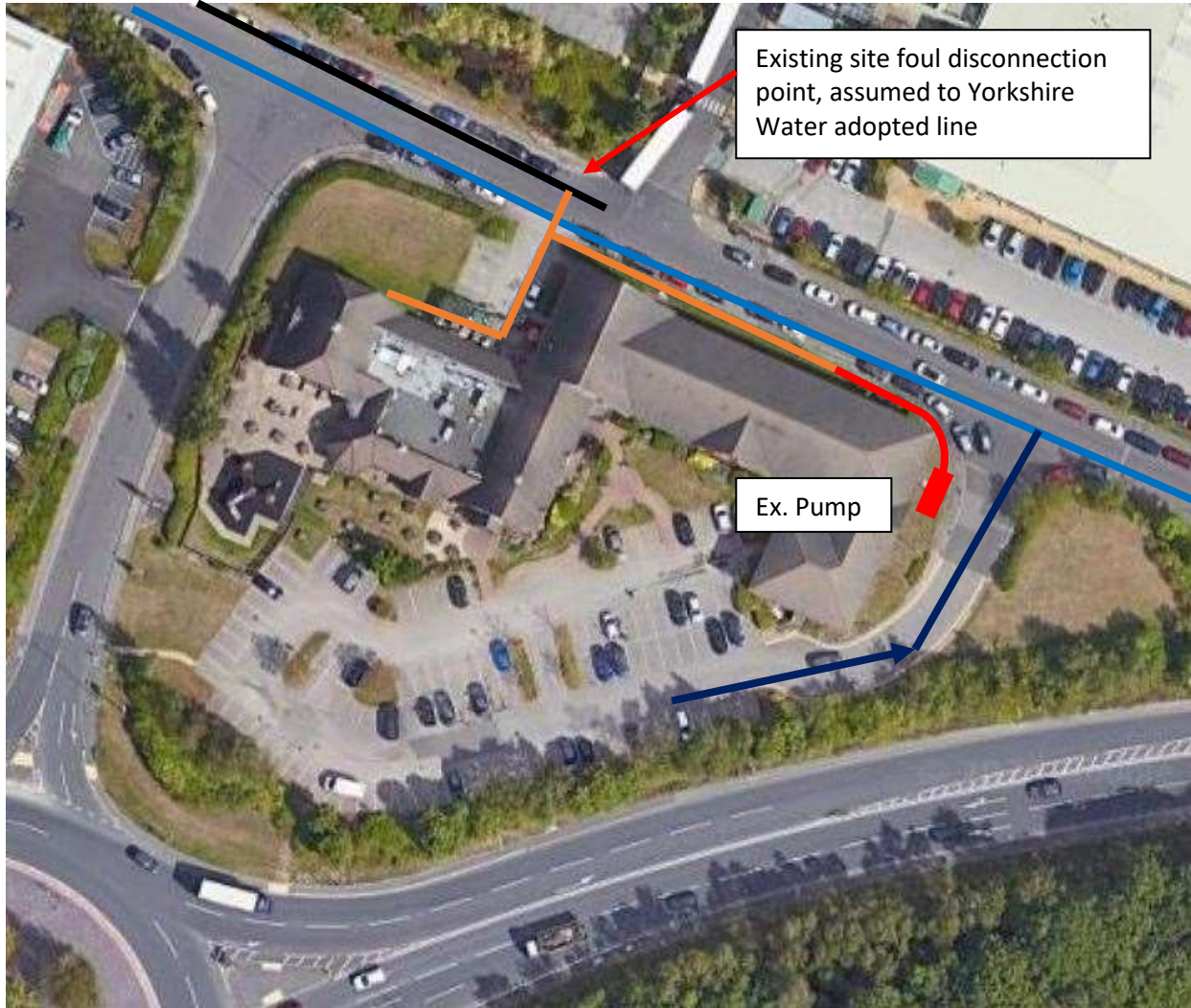
Figure 2. Sewer connection point
