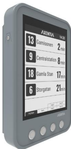
Figure 1: Real Time Passenger Information – Accessible 4-button battery-powered e-Paper display
