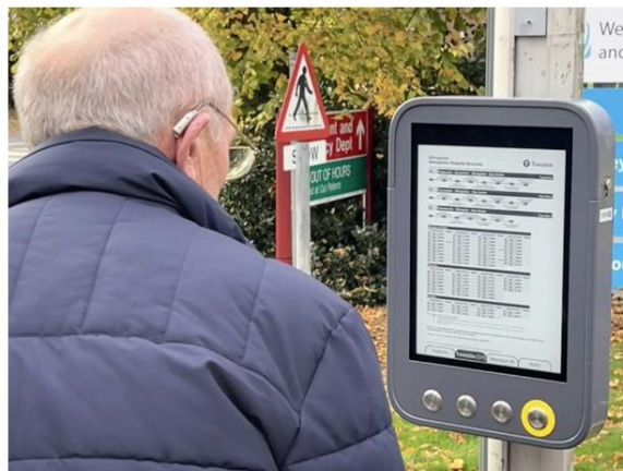
Figure 1: Real Time Passenger Information – Accessible 4-button battery-powered e-Paper display
