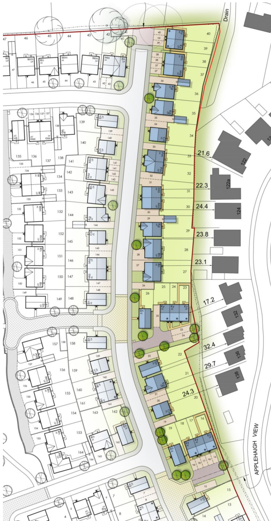
Proposed layout has greater separation distances to existing dwellings along eastern boundary
