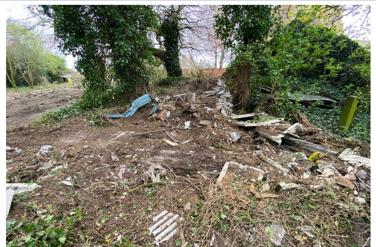
Photograph 5 – ACMs present in the surface soils
