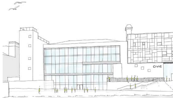
Updated sketch shows the retained floor slab elements breaking up the facade.
