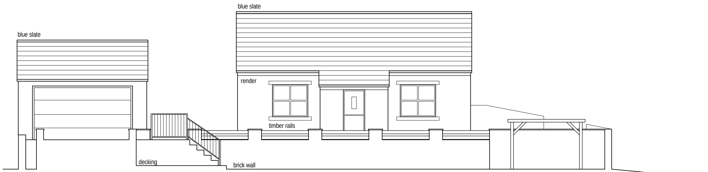
Proposed sectional south facing elevation A - A (1:100)
