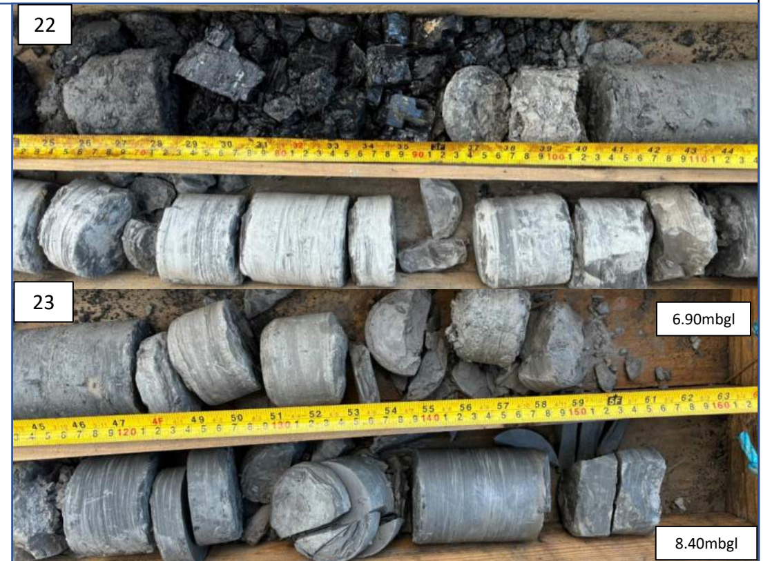
Photograph 22: View of middle third of RC01 cores. 0.20m thick coal seam noted at approximate top depth of 5.80mbgl.
