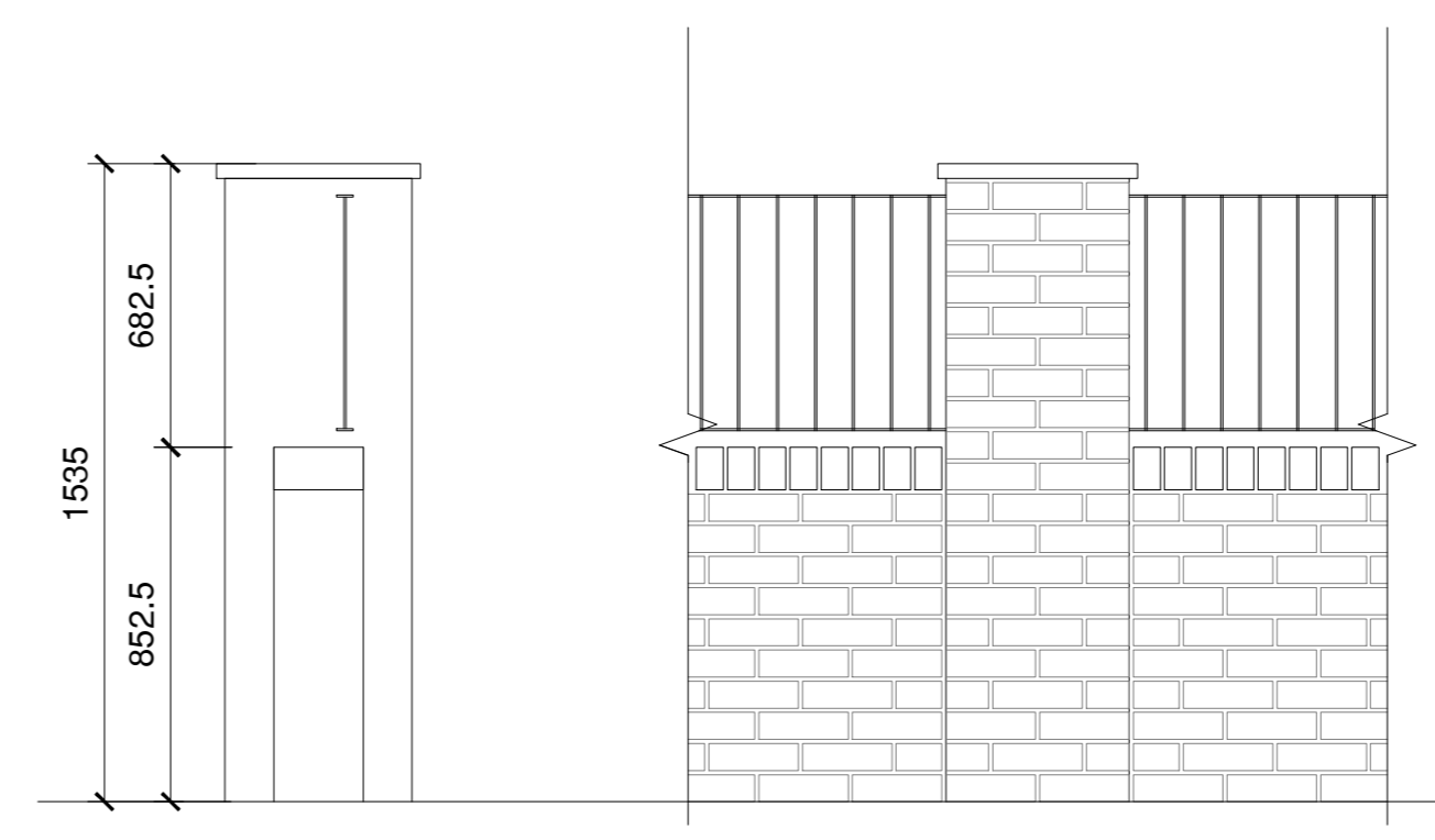
Wall Type D Brickwork piers with artstone capping and 900mm high wall with brick on edge copings. Metal railing fence infill to overall height of 1500mm. Face of railings to sit flush with wall below to prevent climbing
