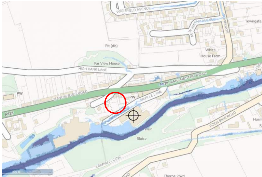
Figure 3 - Surface Water Flood Risk Map
