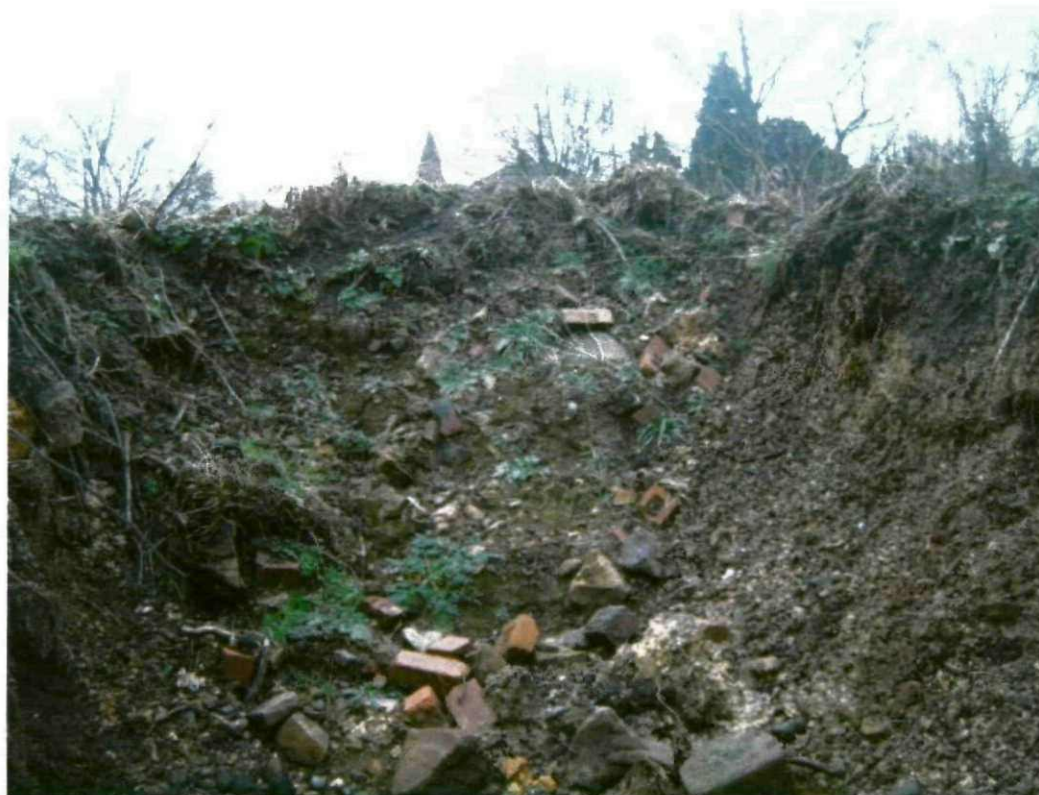
Photograph number 8 showing the soil making material and the coarse rubble which will be screened for the site roads and hard standing.
