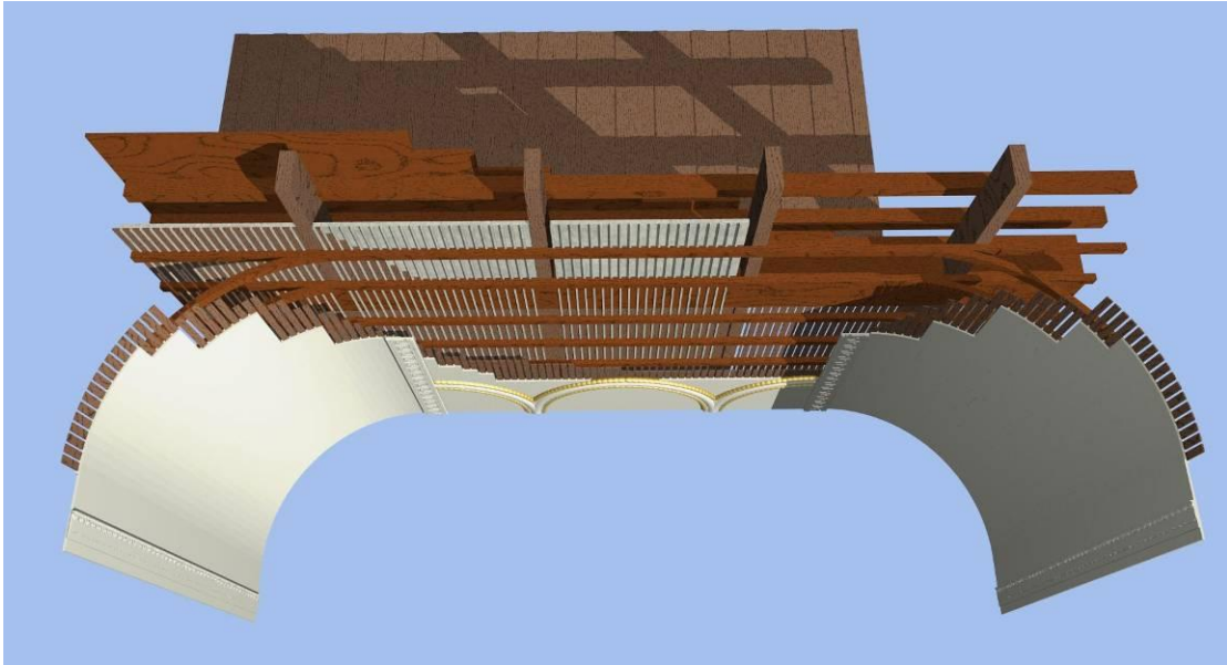
10 Conjectured original construction.
