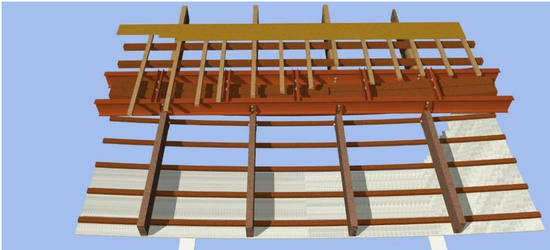
13 Model of proposed structural repair from above.
