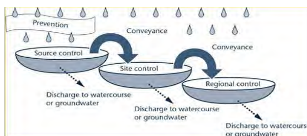
Figure 11 – SuDS Management Train
