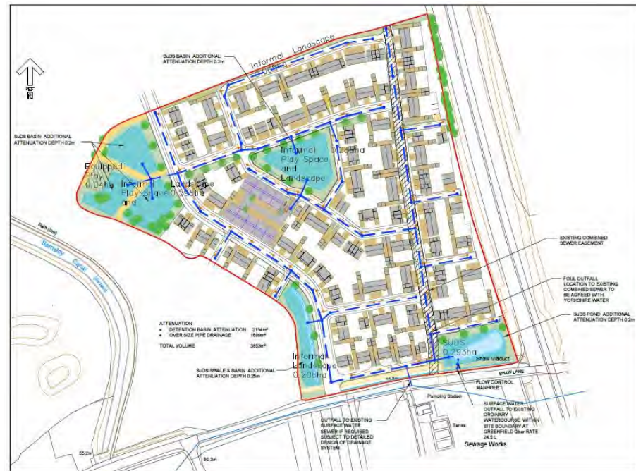
Figure 12 – Indicative Foul Water Drainage Strategy
