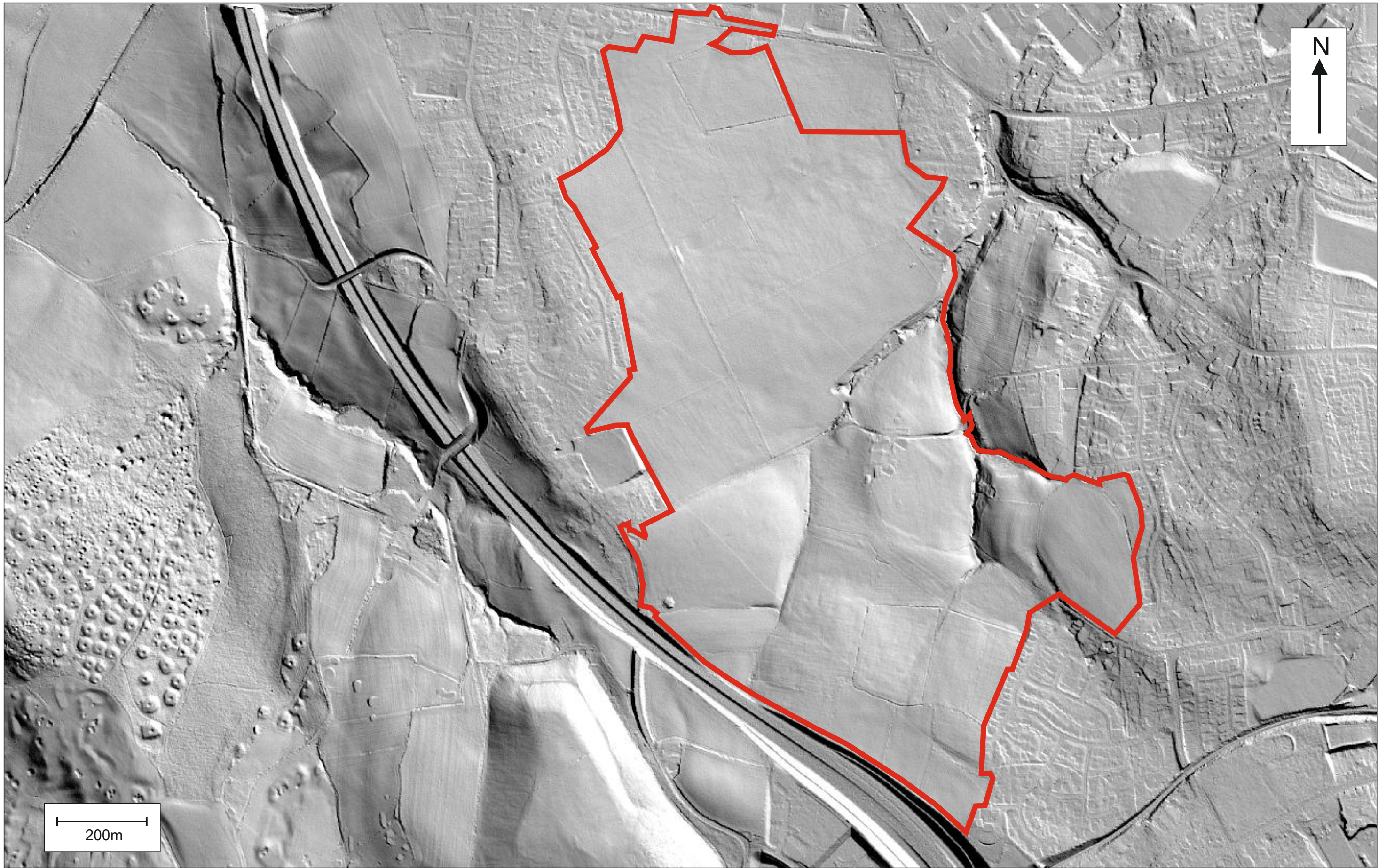
Figure 9.12 Hill-shaded image generated from Environment Agency 1m LiDAR open data
