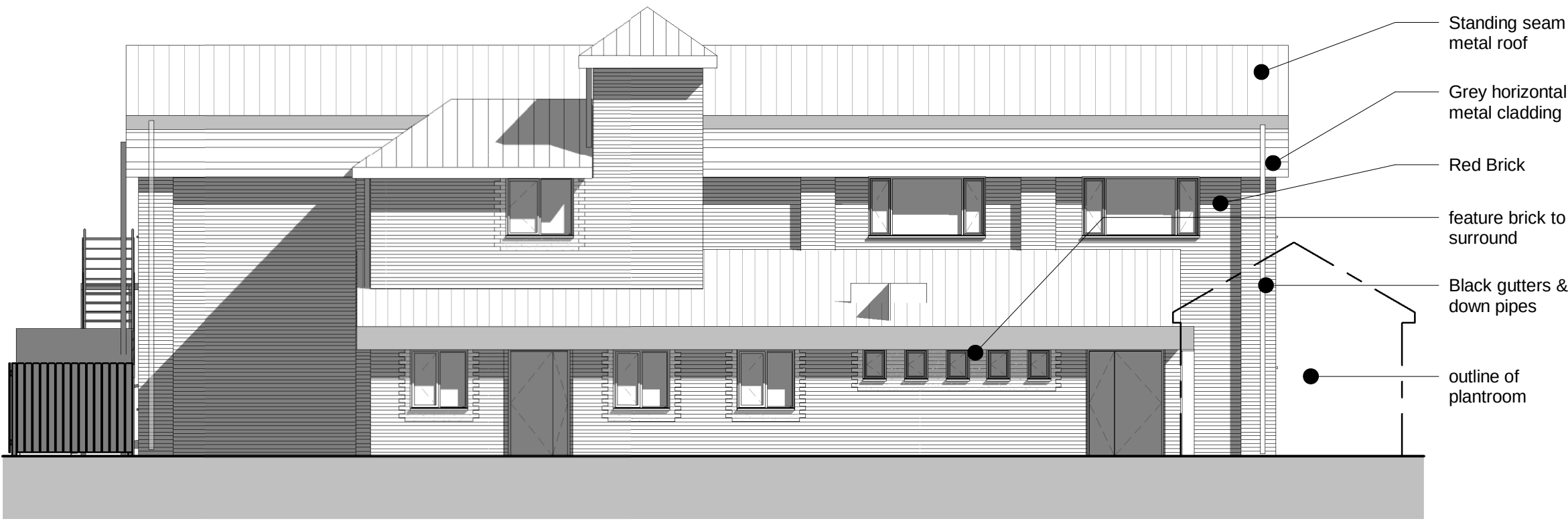
Existing North Elevation 1 : 100
