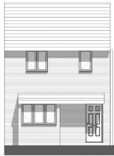
Existing Front Elevation 1:50
