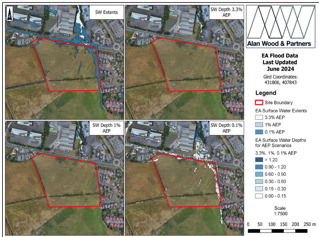
Figure 6: Showing EA surface water flood extents alongside surface water flood depths for varying scenarios.
