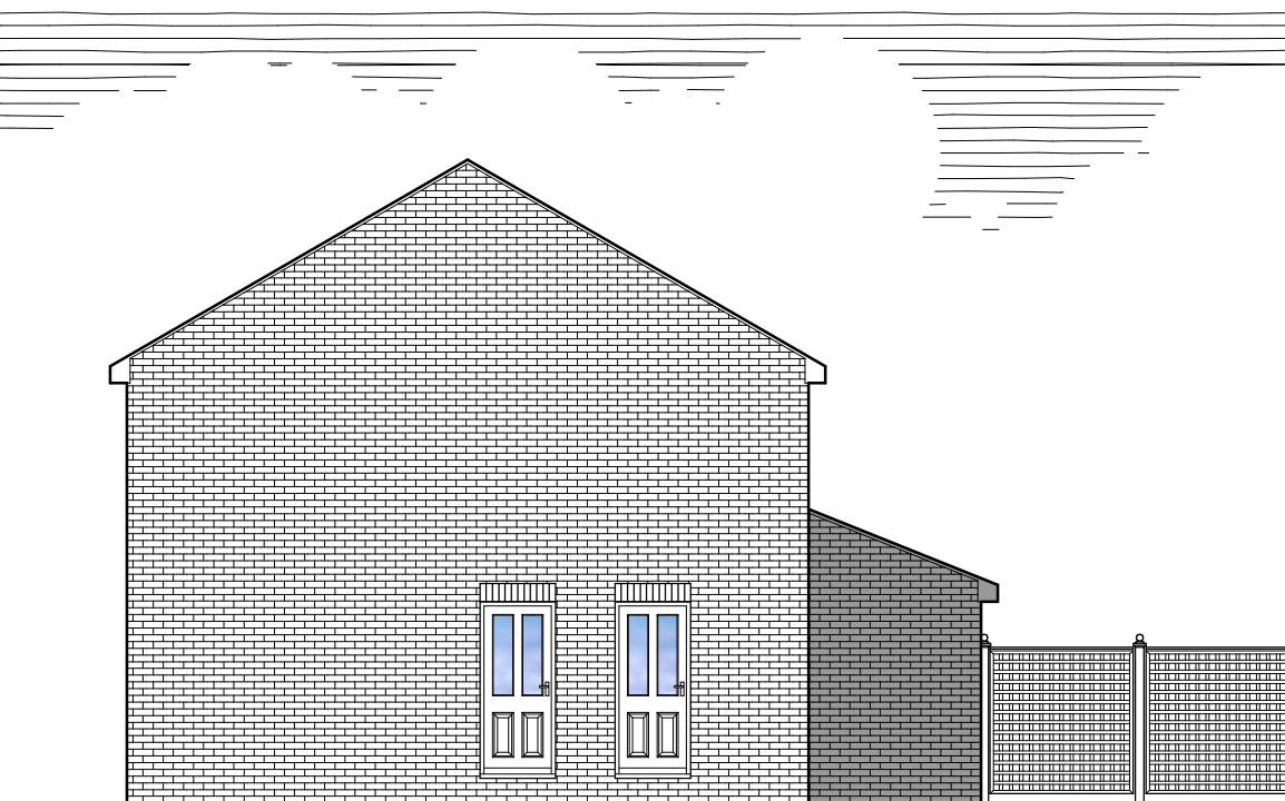
Side Elevation facing adjacent Property as Existing
