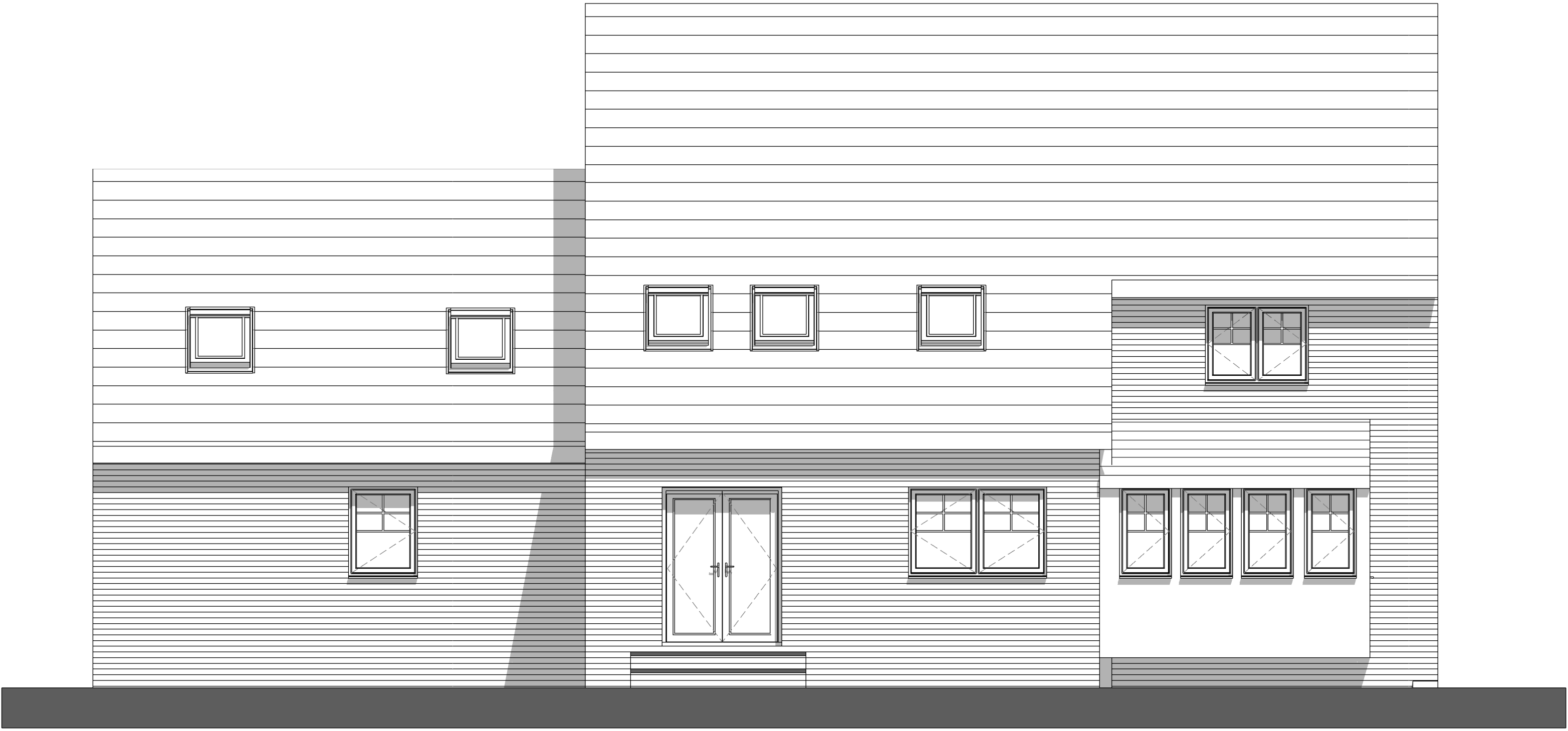
Existing Rear Elevation 1 : 50
