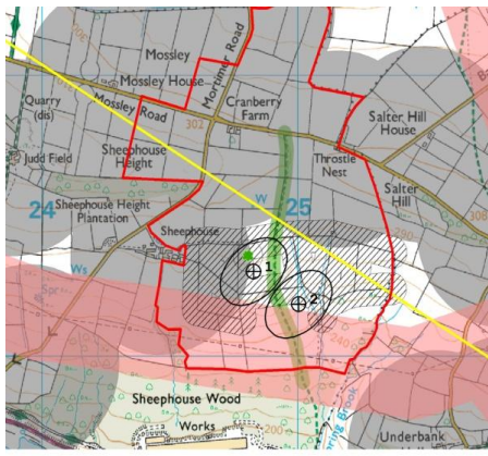
Alternative 4 – Two EWT-DW54 Turbine (80m to tip; 54m diameter blade; total 1.8MW)
