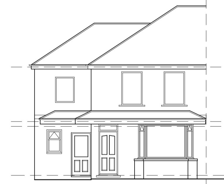
EXISTING FRONT ELEVATION SCALE 1:100
