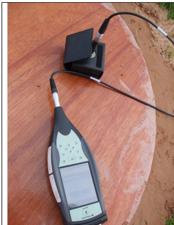
Figure 16 – Calibrating Sound Monitor
