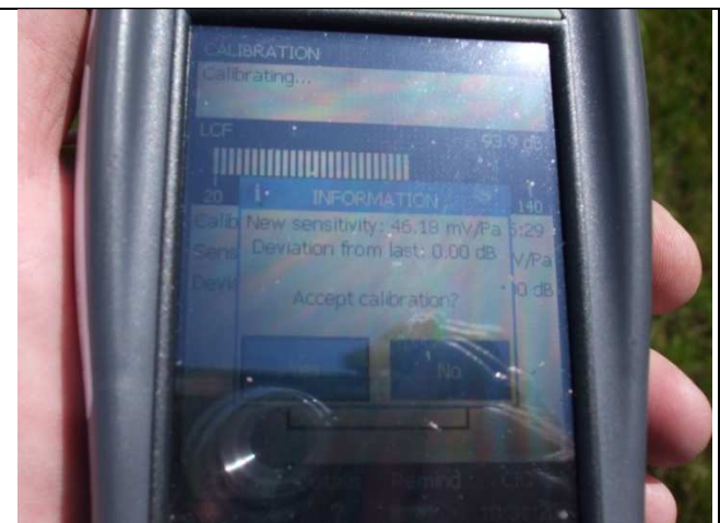
Figure 8 – Sound Monitor Calibration Result
