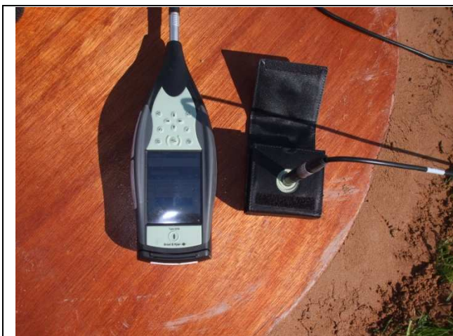
Figure 7 – Calibrating Sound Monitor
