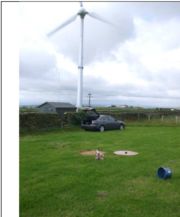
Figure 5 – Using Damp Sand to Mount Sound Board
