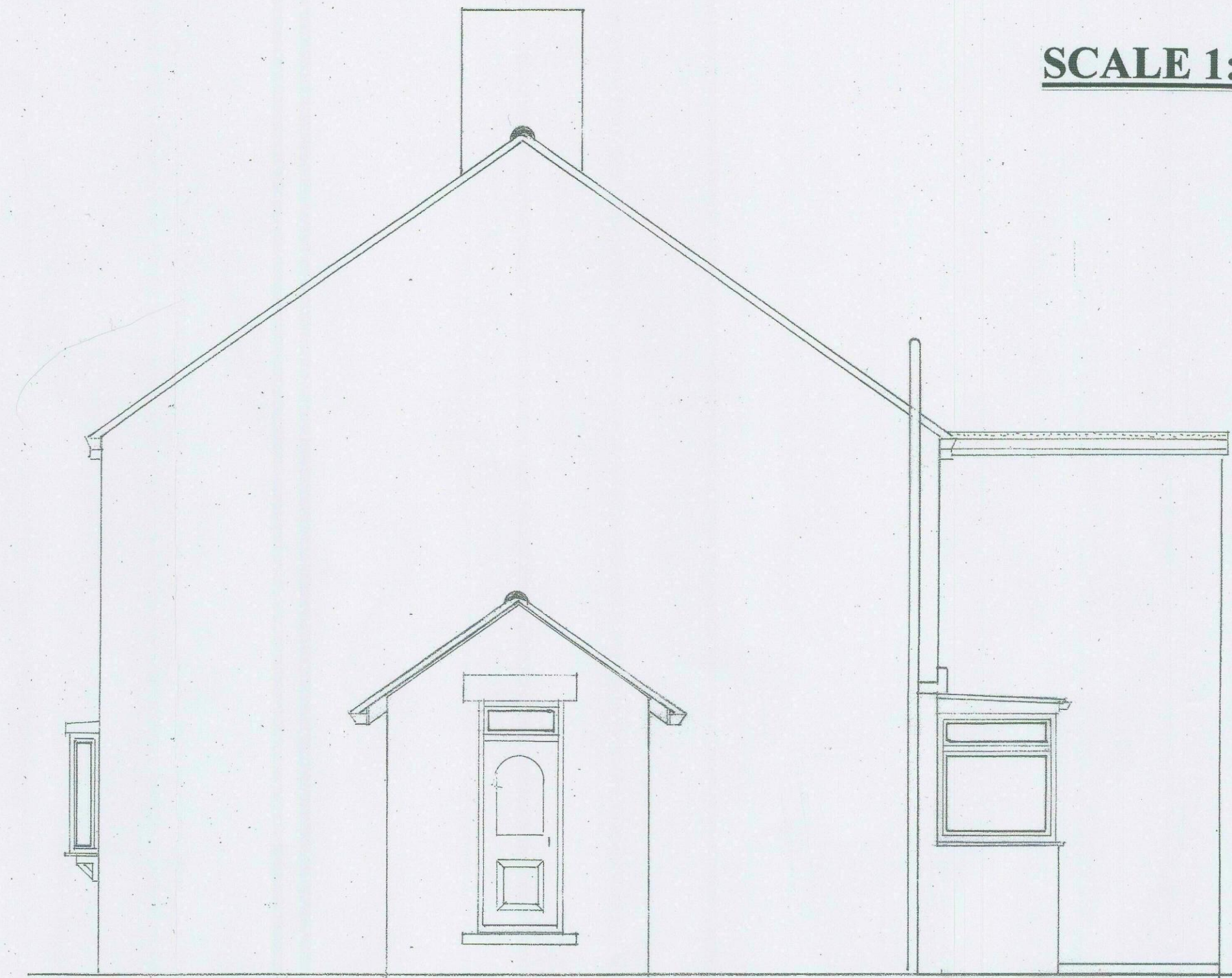
EXISTING SIDE ELEVATION A
