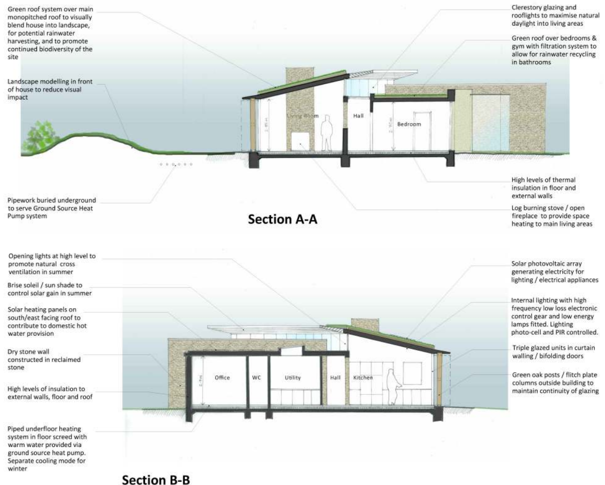
Figure 10 - Concept sections showing possible use of low/zero carbon & renewable technologies in servicing the building
