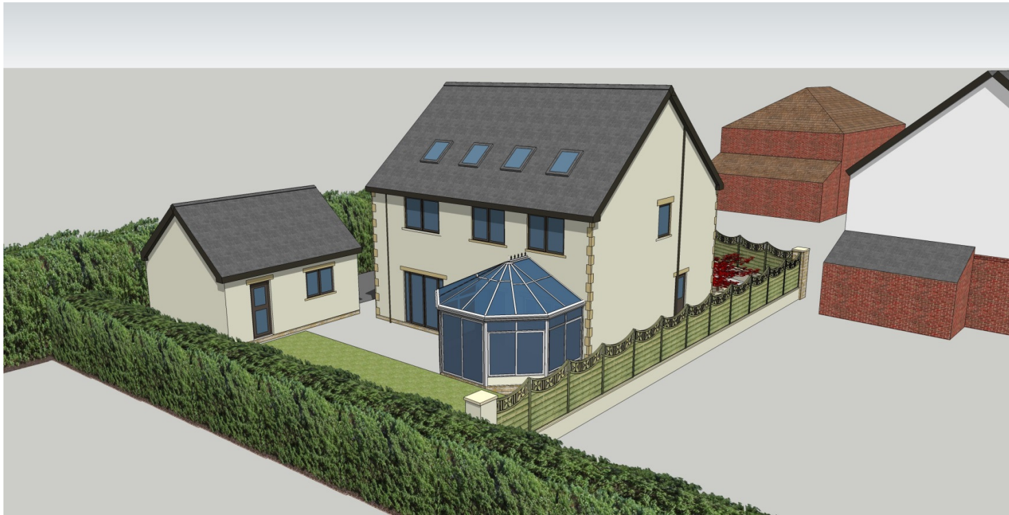
Aerial view of south and west elevations, note the side elevation of the conservatory is now to be solid rendered masonry, in line with the planning officers comments.
