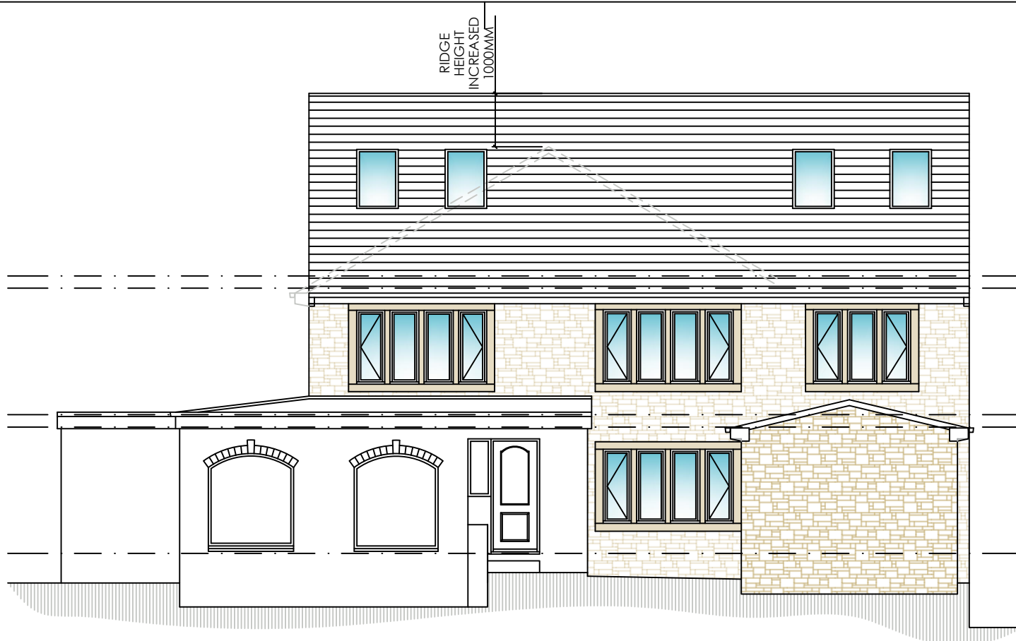
PROPOSED SOUTH ELEVATION SCALE 1:100
