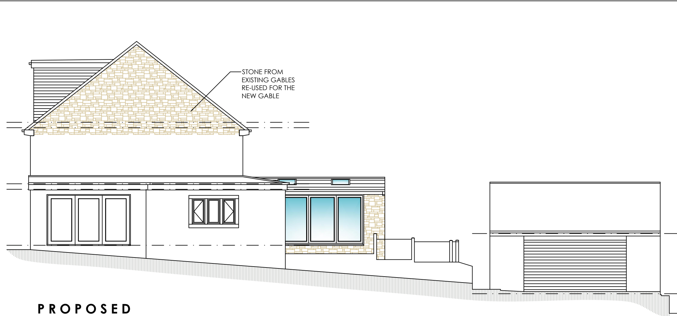
PROPOSED WEST ELEVATION SCALE 1:100
