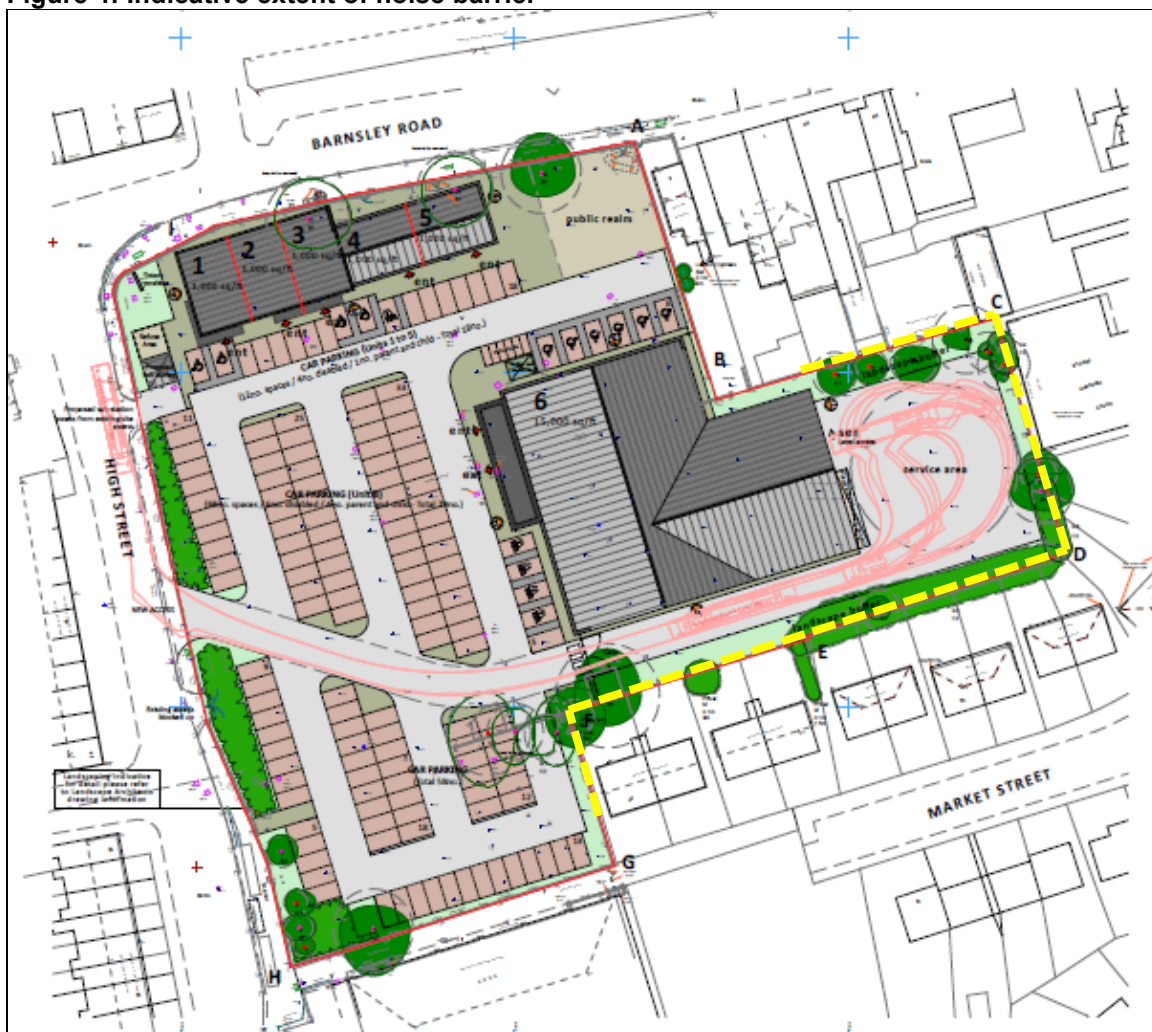
Figure 4: Indicative extent of noise barrier
