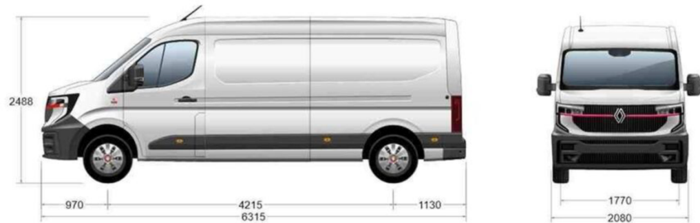
Figure 1 Typical 3.5t extra-long wheelbase van
