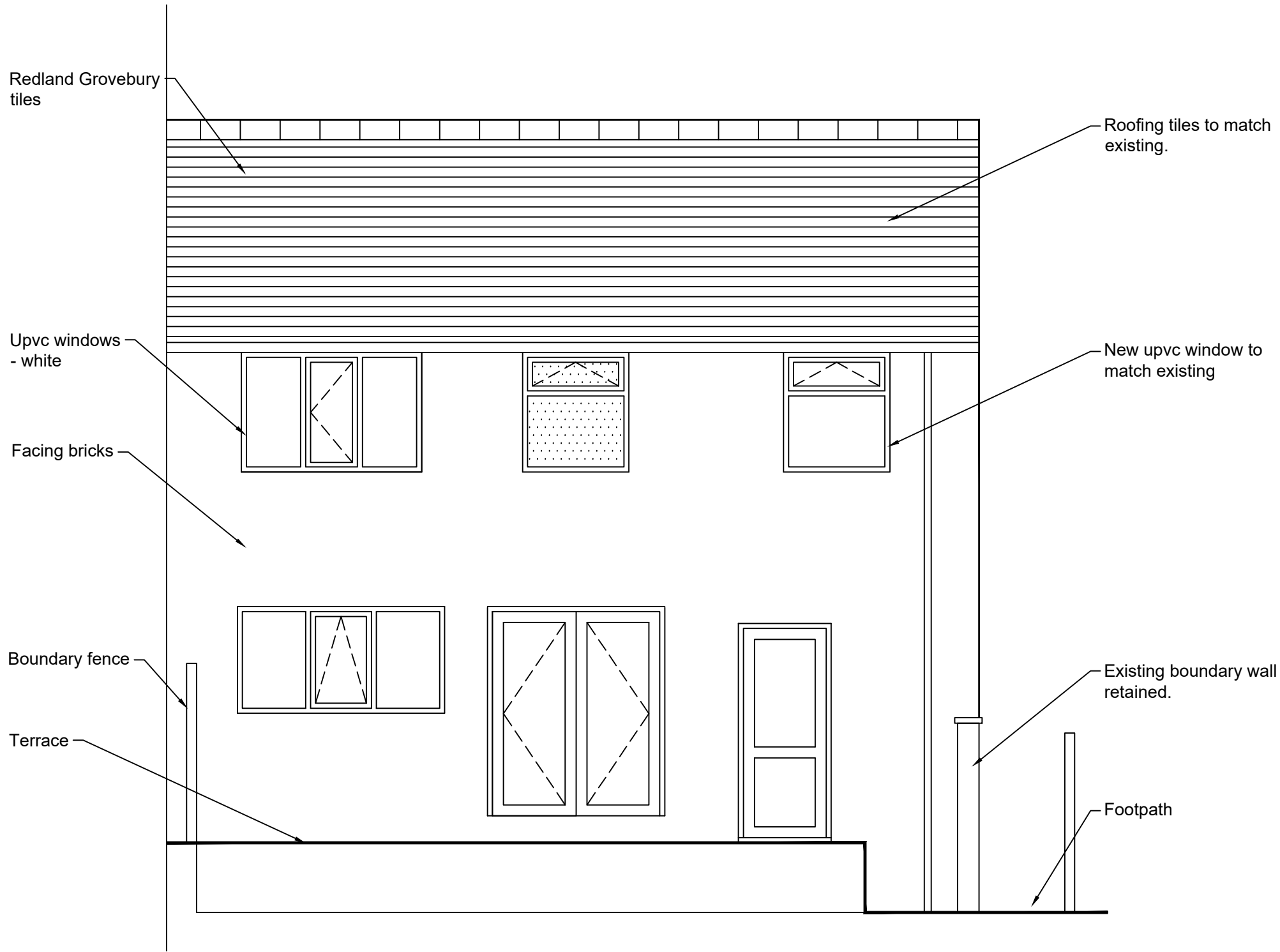
PROPOSED REAR ELEVATION 1:50
