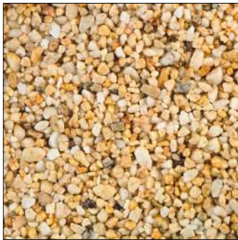
Permeable resin bond gravel.
