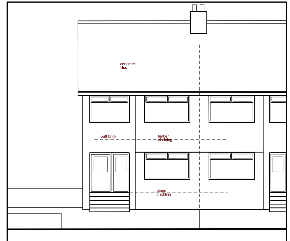
North Elevation - Existing
