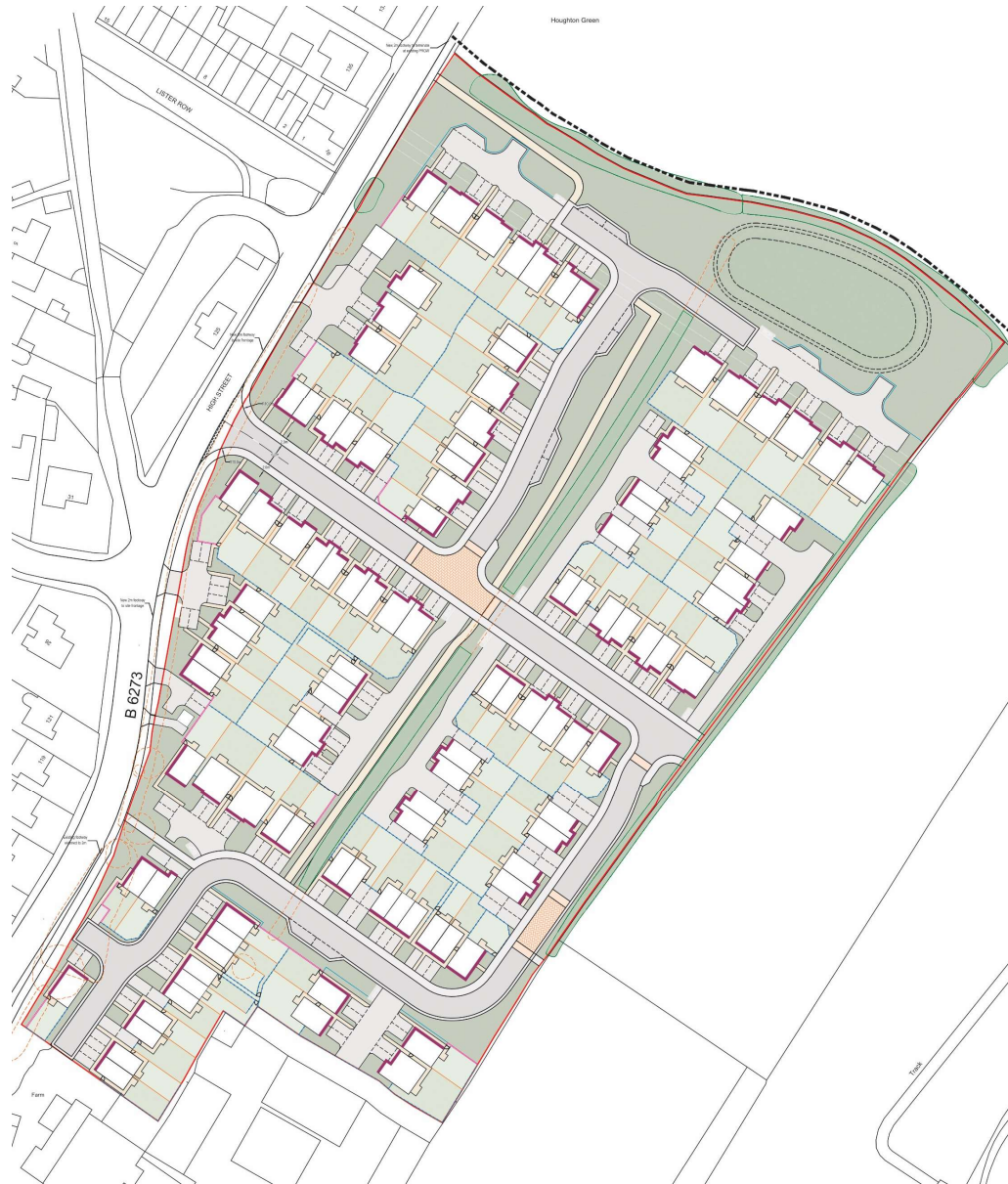
Proposed plan showing the active frontages of the designed scheme to help design out crime.
