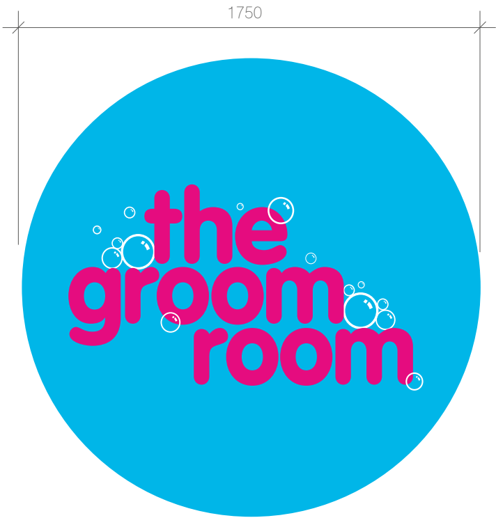
Item 4 1No Internally illuminated Roundel Sign. Aluminium returns with acrylic face. Size: 1750mm Scale: 1:50
