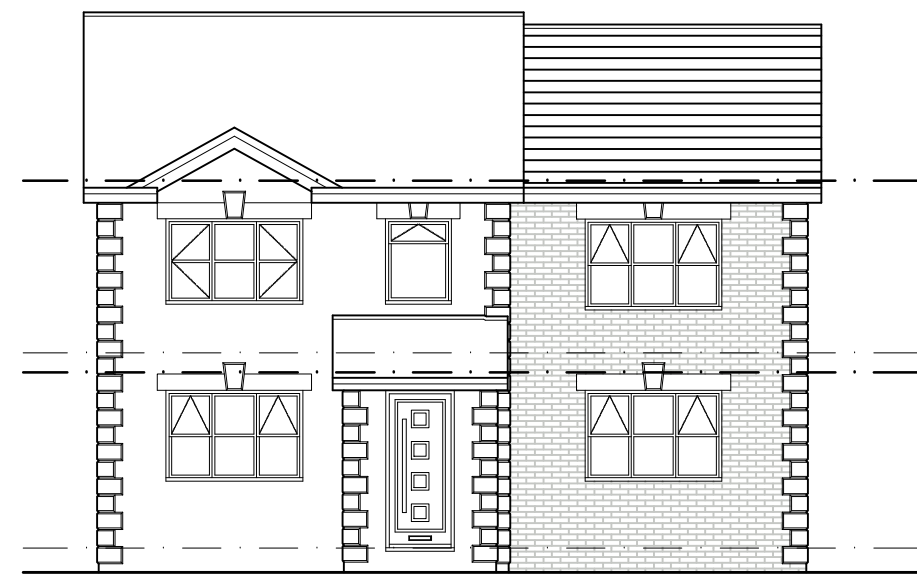
PROPOSED FRONT ELEVATION SCALE 1:100
