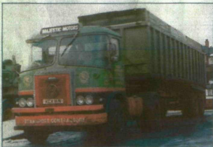
What a sound this beast must have made - Atkinson Borderer had a straight-eight Gardner 240 engine.
