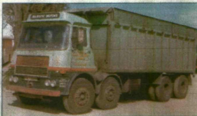
Harry Cawthorne was originally convinced that this ERF A-series would not cope with colliery stacking yards, but it turned out to give sterling service.
