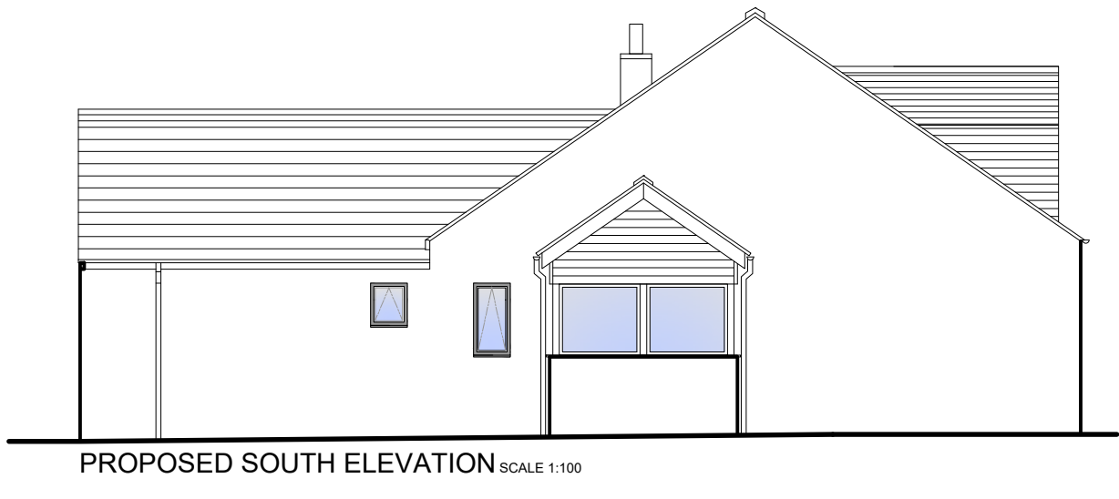
PROPOSED SOUTH ELEVATION SCALE 1:100
