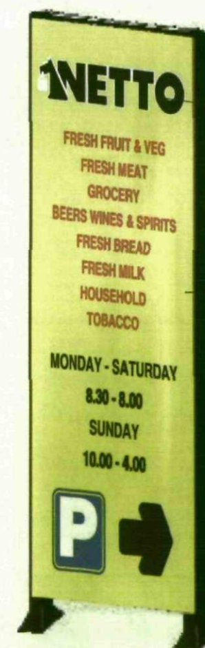
TOTEM SIGN 1500MM WIDE X 5000MM HIGH X 200MM DEEP TOTEM SIGN COMPRISING: YELLOW ROLLED PANELS MOUNTED ON BLACK TUBES WITH WELDED BASE PLATES. NETTO LOGO BUILT UP USING 5MM ALYOGLAS 10021003 ACRYLIC 500MM HIGH WITH WITH 100MM RETURNS. ILLUMINATED BY MEANS OF WHITE LED'S, BLACK VINYL TO FACE LEAVING BORDER AND RETURNS ILLUMINATED. ALL LETTERING AND OTHER IN VINYL.
