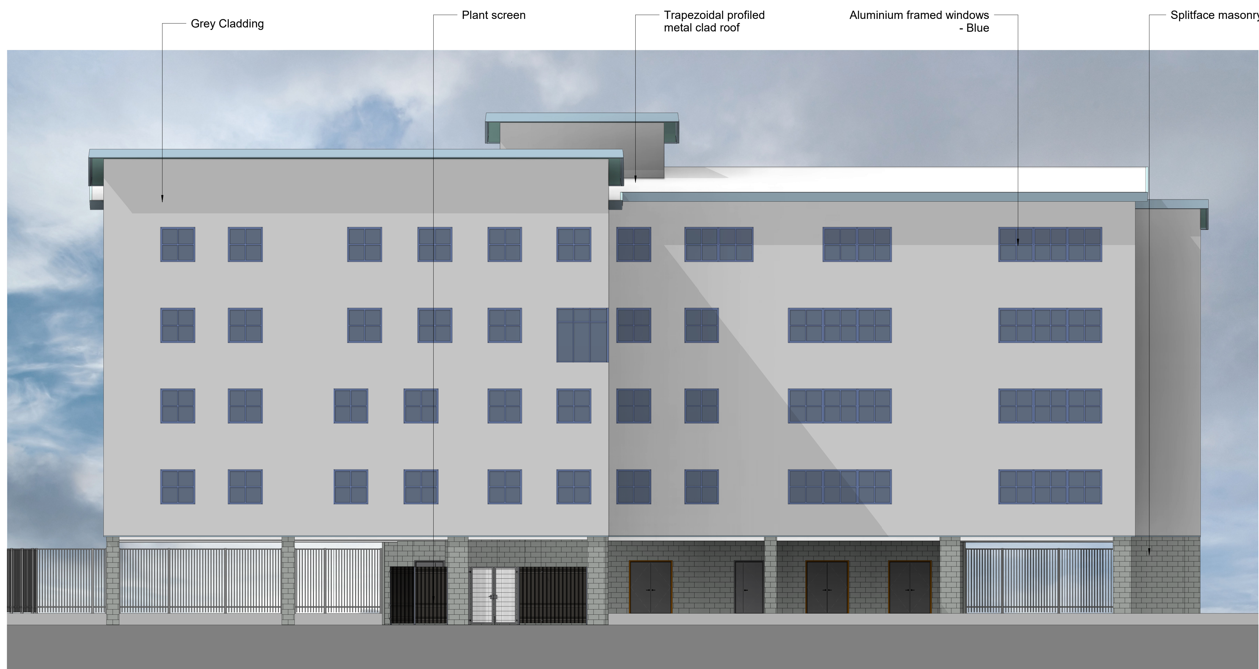
Existing East Elevation
