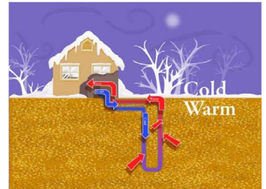
Ground Source Heat Pump
